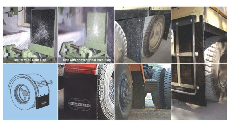
Spray Suppression System (3S) Rainflaps designed by Time Technoplast Ltd. (TIME) is a perfect answer. These flaps consist of a unique surface formed by multiple tufts / grass blades with a strong and sturdy backing. This surface contains the water spray and reduces the pulverization of water thus limiting formation of water spray. It absorbs the kinetic energy and guides the water downwards.
